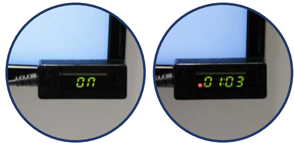
Display with integrated IR. Displays channel (ON) and time (OFF)
