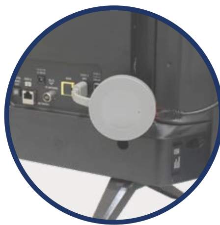
CR 4K device connected to a television and a wired LAN network
