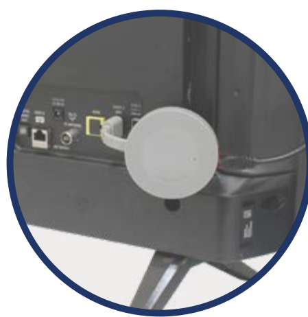
CR 4K device connected to a television and a wired LAN network
