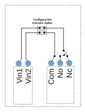
**Attention**: Please note that the CCA+ can be powered regardless of the input polarity, but the output Com terminal is connected to the Vin2 input and the No/Nc to the Vin1.
