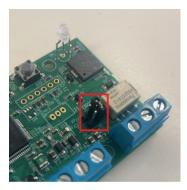
For this configuration, you only have to connect the Jumper in a vertical position as indicated in the
