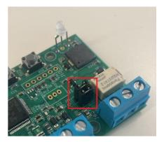
The Jumpers must be connected horizontally, as shown in the following diagram:
