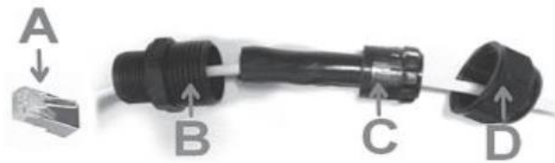
Figure 3-16 Wrapping Waterproof Materials Around Ethernet Cable
