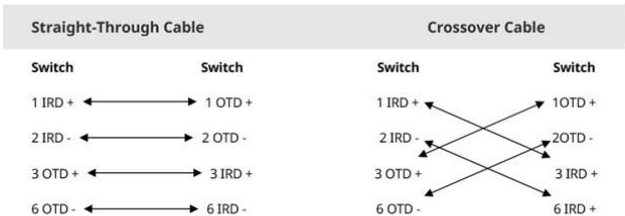
Figure 7-3 100BASE-TX/10BASE-T Twisted Pairs Connection
