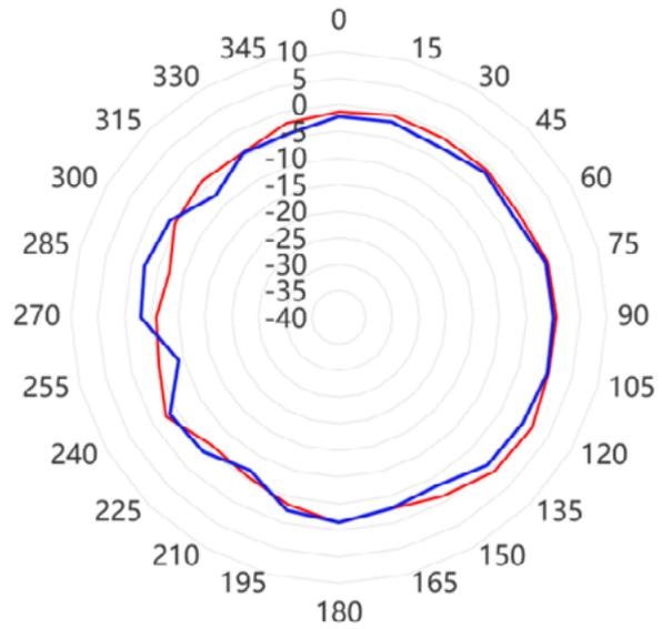
— 5 GHz Azimuth Plane Theta=60°
