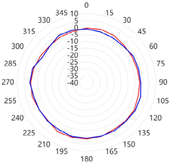
— 2.4 GHz Azimuth Plane Theta=60°
