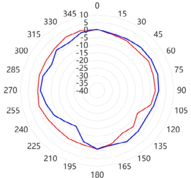
— 5 GHz Azimuth Plane Phi=0°
