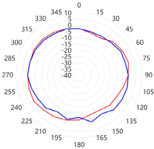
— 2.4 GHz Azimuth Plane Phi=0°
