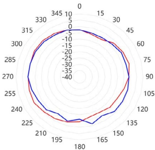
— 2.4 GHz Azimuth Plane Phi=0°
