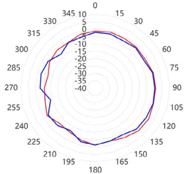
— 5 GHz Azimuth Plane Theta=60°
