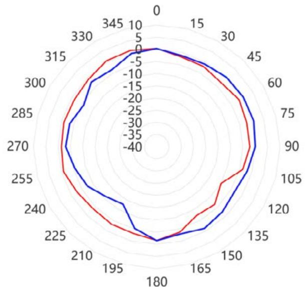
— 5 GHz Azimuth Plane Phi=0°
