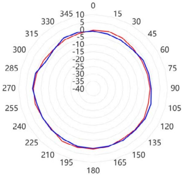
— 2.4 GHz Azimuth Plane Theta=60°
