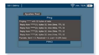
It allows to detect and connect to WiFi 2.4GHz networks, see the power of each network and make tests of the link to the network (PING).
