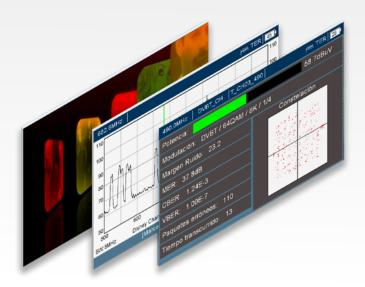
Fast switching between spectrum, measurements and image. By pressing the button of the desired mode, each functionality is quickly accessed. The dynamic navigation mode allows access to each channel as programmed.
