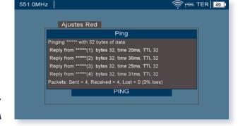
It allows to detect and connect to WiFi 2.4GHz networks, see the power of each network and make tests of the link to the network (PING).
